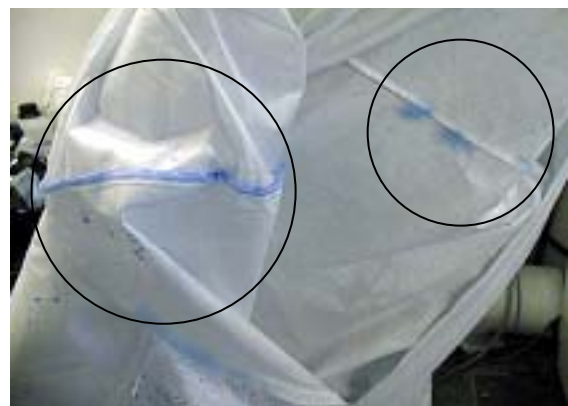
Figure 4: Poor finish detected by spray test, photo: Sächsisches Textilforschungsinstitut e.V. – Chemnitz (Saxon Textile Research Institute, registered association, in Chemnitz)
