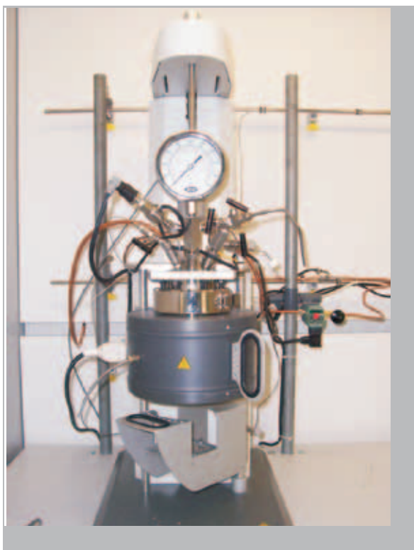
Abb. 11: Foto des Edelstahlrührreaktors – Photo of the stainless steel stirred tank reactor
