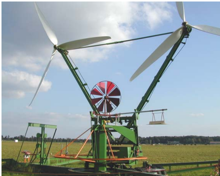
Figure 4.18: Lee-wind wheel in storm position for MoWEC safety.
