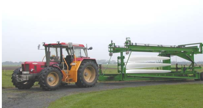
Figure 3.21: MoWEC during transportation. MoWEC während des Transportes.
