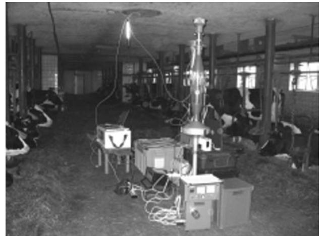
Figure 6: Set of instruments to measure concentration and particle size inside the stable
