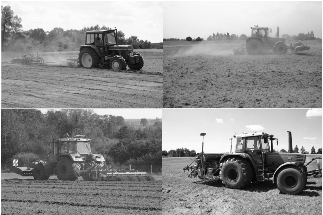
Figure 2: Investigated agricultural operations: plowing including a packer, harrowing, disking, and cultivating
