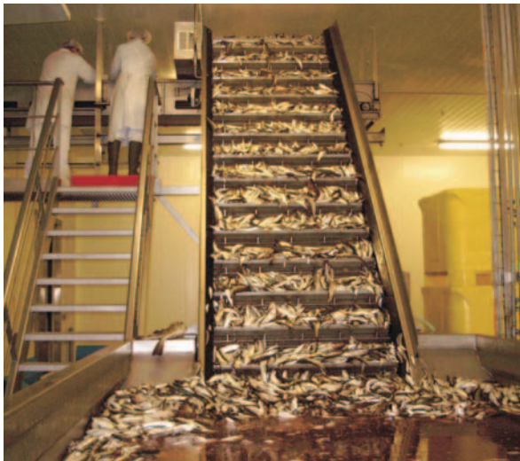
Abb. 10: Transport des Fanges in die Sortieranlage - Transport of fish to the grading equipment.
