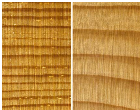
Figure 4: Macroscopic structure of softwoods. (left): transverse plane of spruce with the occurrence of resin canals. (right): transverse plane of white fir without resin canals
