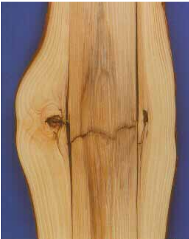
Fig. 10: Tangential view of „Wulstholz“ formation in a spruce tree. Note the compression damage in the regular wood tissue and discolouration by fungal infection.
