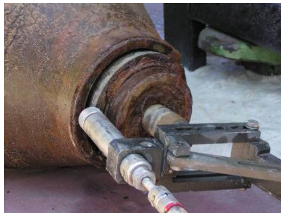
Fig. 4: Defusing of a GP 500 bomb using remotely controlled water abrasive suspension cutting © ANT AG, Lübeck, Germany
