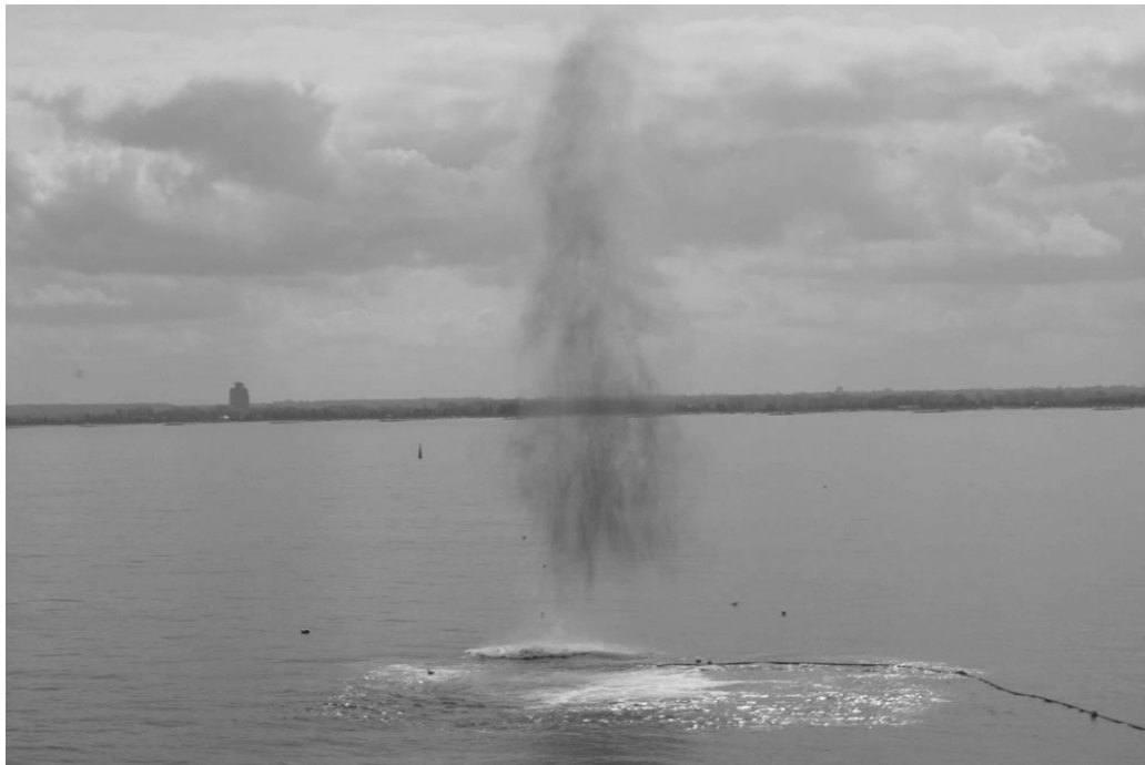
Fig. 1: Test detonation when using a bubble curtain
