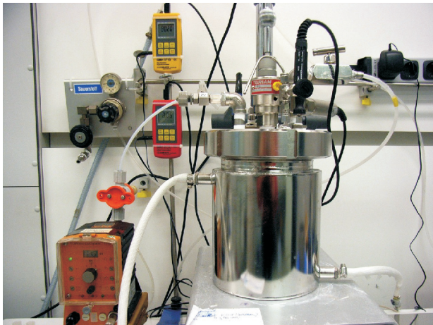
Abb. 11: Edelstahlreaktor zur Glucoseoxidation – Stainless steel pressure vessel for glucose oxidation
