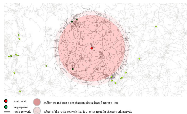
Figure 2: Method of catchment area analysis prior to the routing analysis.
