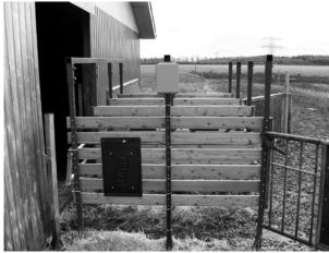
Figure 3. Gates with RFID scanner
