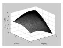
Fig.7 Temperature of the middle layer on the 5th day
