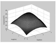
Fig.8 Temperature of the middle layer on the 10th day
