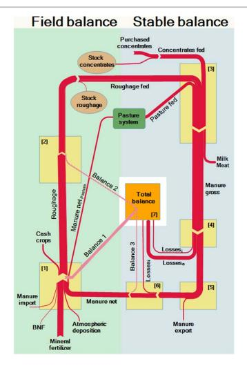
**Figure 1.** Example of nitrogen flow analysis for a dairy farm. Boxes 1–7 indicate points of even mass balances for nitrogen (own design following the sample representation in Schüler *et al* 2016).
