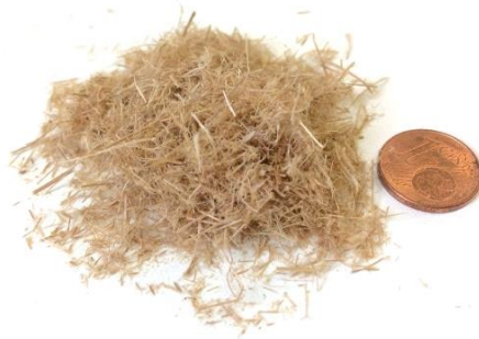
Figure 11: RM pulp produced with atmospheric pressure from Ethiopian highland bamboo (Kickhöfen 2019)
