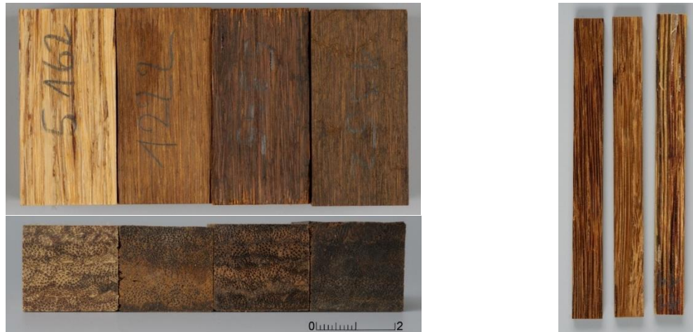
Figure 77: Top view and cross section (left) of specimens tested against basidiomycetes from samples made from heat treated bamboo scrimber (Ctrl, 160, 180, 200 °C) and specimens from surface layer and core layer (right)
