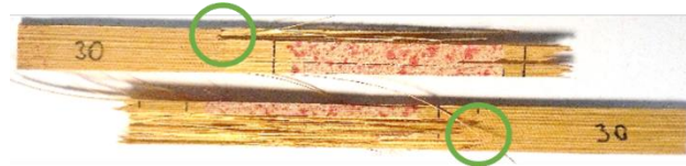
Figure 48: Interlaminar shear and fiber pullout in a tension loaded bamboo internode sample with a high FBD indicating the initial location of failure occurred at the specimen clamping edge
