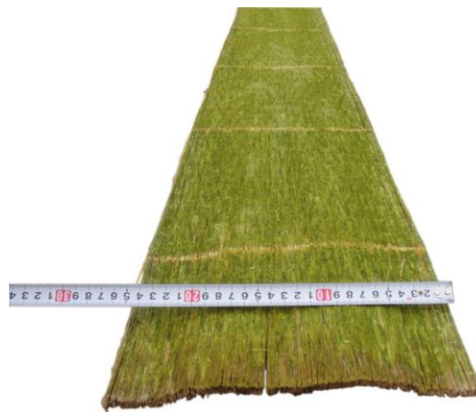
Figure 24: Bamboo scrim produced in a 4 th generation fluffing machine comprising the epidermal green part of moso (Yu et al. 2014a)
