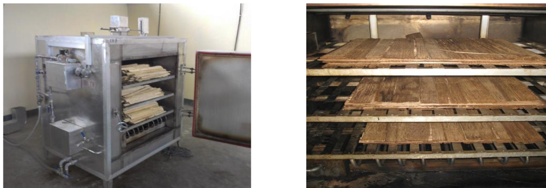
Figure 56: The lab-scale kiln chamber (left) and treated strands after 3 h / 160 °C (right)
