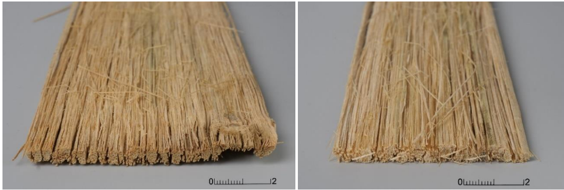
Figure 68: Scrim strands from the top portion (left) and fine crushed scrims from the same top portion (right)
