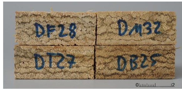
Figure 102: Cross section of scrimber specimens made from crushed scrims coming from bottom (B), middle (M), top (T) portion of the culm and a finer crushed (F) variant
