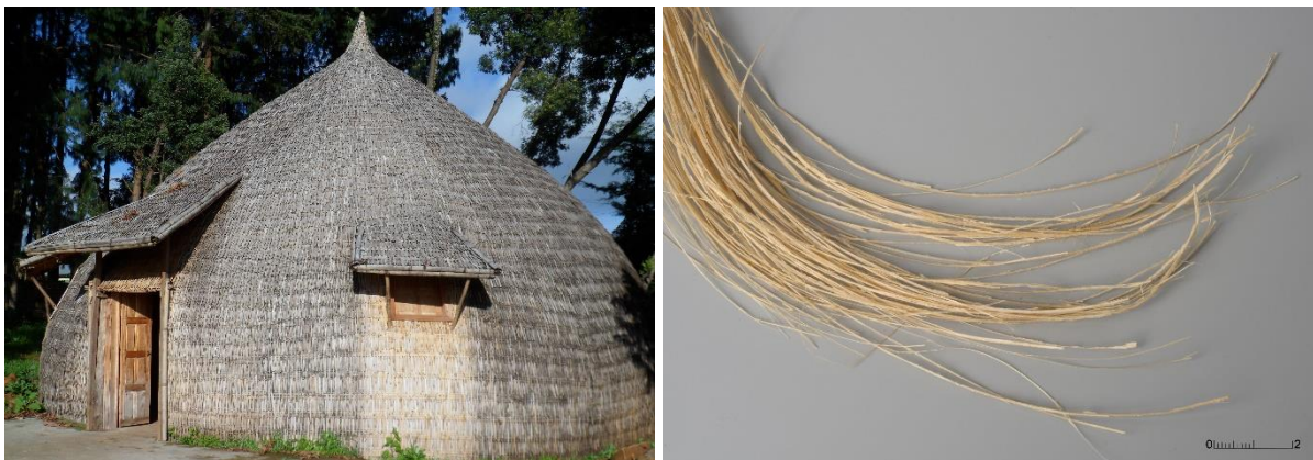
Figure 8: Traditional Sidamo dome house made from woven bamboo strips (left) and mechanically extracted technical bamboo fiber (right)
