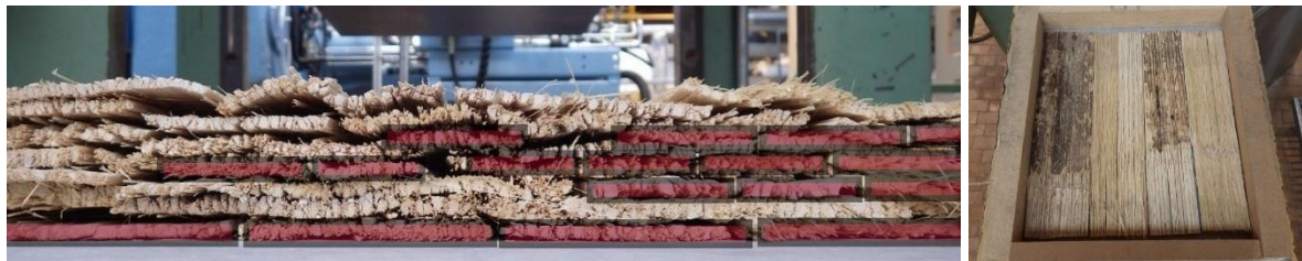
Figure 58: Mat formation with narrow scrims in the core, medium strands in the center and broad strands in the face layer (left) using a softboard template (right)
