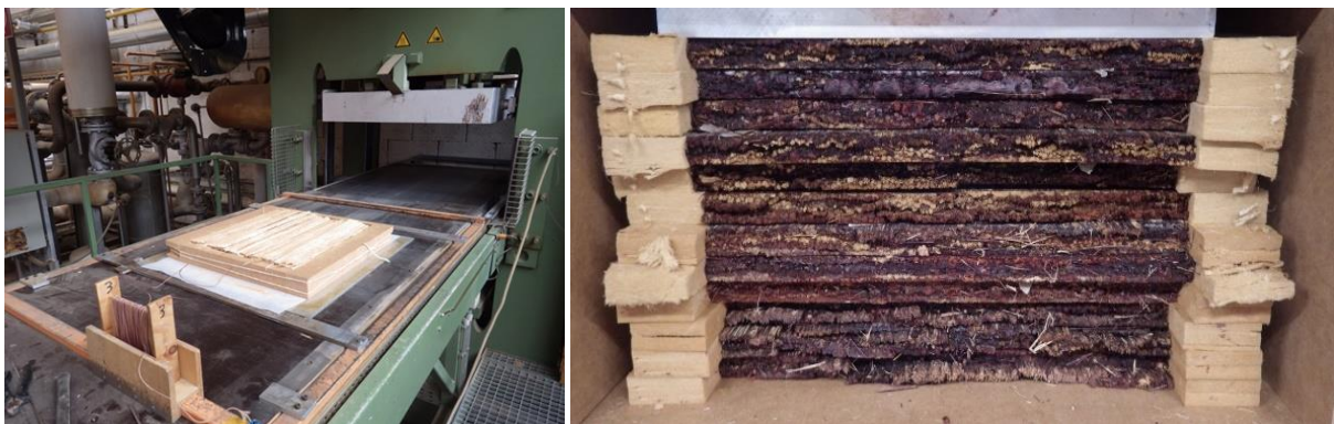
Figure 59: Press-ready fiber bundle mat with a temperature probe in the core layer (left) and conditioning in a warm veneer press forming a hot stack for curing (right)
