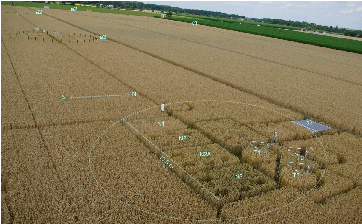
FIGURE 1: View of the trial field with three circular main plots at ambient (a1–a3) and at elevated CO 2 (e1–e3). In the foreground the ambient ring a3 with the spatial arrangement of four subplots (3 m x 5 m) with different N supply (N1, N2, N3; N2A) and the three hexagonal arrays (diameter 1.3 m) with heaters for the warming treatments (T1, T2) and with dummies (T0) is shown.
