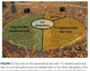
**FIGURE 1** Top view on the experimental area with <sup>19</sup>C-labelled beech leaf litter on one half (yellow) and non-labelled litter on the other half (green) of the area surrounding each of the three accessible soil observatories (Ø 150 cm). The experimental areas directly adjacent to the soil observatories have a radius of 150 cm.
