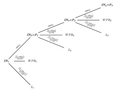
Fig. A.1. Tree diagram on wood resource input and output, conversion efficiency, WPR and losses.
