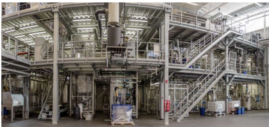
YXY® Technology pilot plant in Geleen, The Netherlands consisting of an SDH unit for MMF, an oxidation unit for cFDCA and a purification unit to produce pFDCA. [Avantium]
