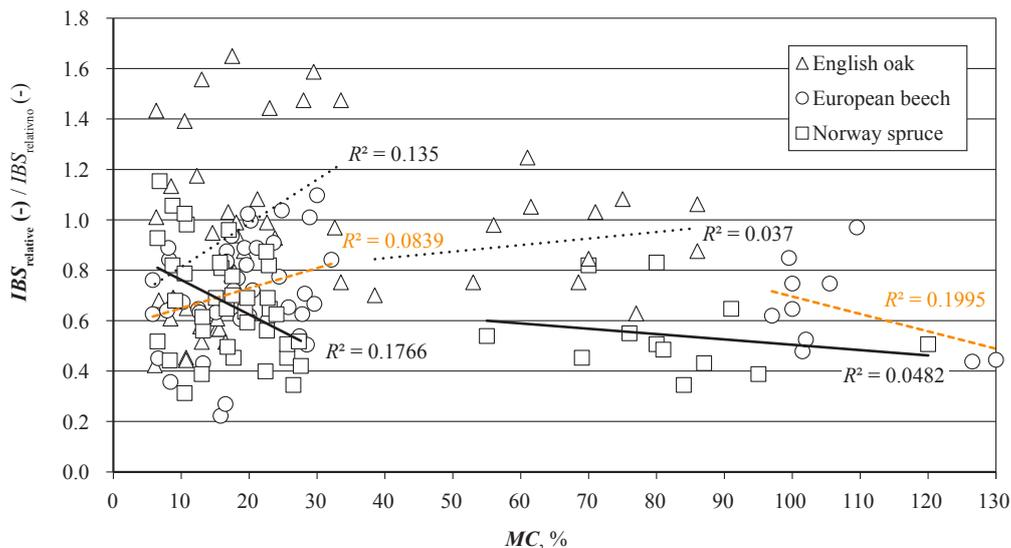
**Figure 4** Relative impact bending strength ( $IBS_{relative}$ ) depending on MC in hygroscopic and over-hygroscopic MC range shown for English oak (*Quercus robur* L.), European beech (*Fagus sylvatica* L.) and Norway spruce (*Picea abies* (L.) H. Karst.)
