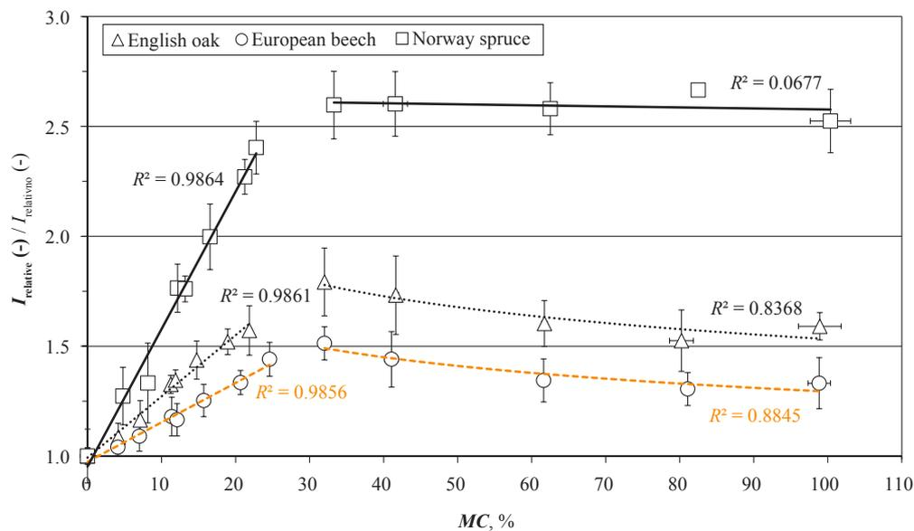
**Figure 1** Relative degree of integrity ( $I_{relative}$ ) depending on MC in hygroscopic and over-hygroscopic MC range shown for English oak (*Quercus robur* L.), European beech (*Fagus sylvatica* L.) and Norway spruce (*Picea abies* (L.) H. Karst.)
