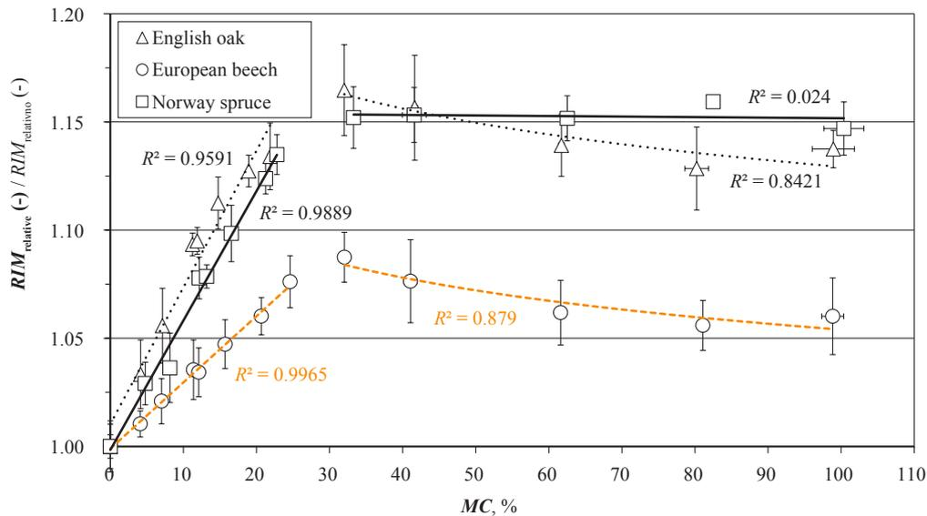
**Figure 3** Relative resistance to impact milling ( $RIM_{relative}$ ) depending on MC in hygroscopic and over-hygroscopic MC range shown for English oak (*Quercus robur* L.), European beech (*Fagus sylvatica* L.) and Norway spruce (*Picea abies* (L.) H. Karst.)
