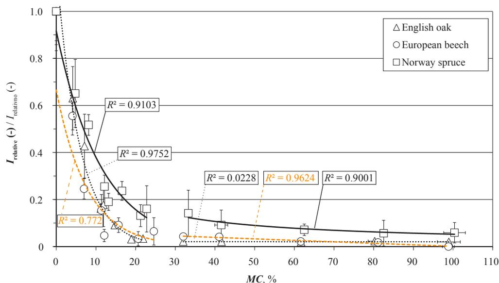
**Figure 2** Relative fine fraction ( $F_{relative}$ ) depending on MC in hygroscopic and over-hygroscopic MC range shown for English oak (*Quercus robur* L.), European beech (*Fagus sylvatica* L.) and Norway spruce (*Picea abies* (L.) H. Karst.)
