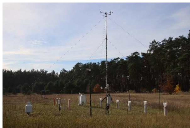
Figure 5-1: Throughfall samplers on a Level II plot (left) and open-field samplers on a neighboring meadow (right) in Schorfheide, Germany (Images: Berit Michler)
