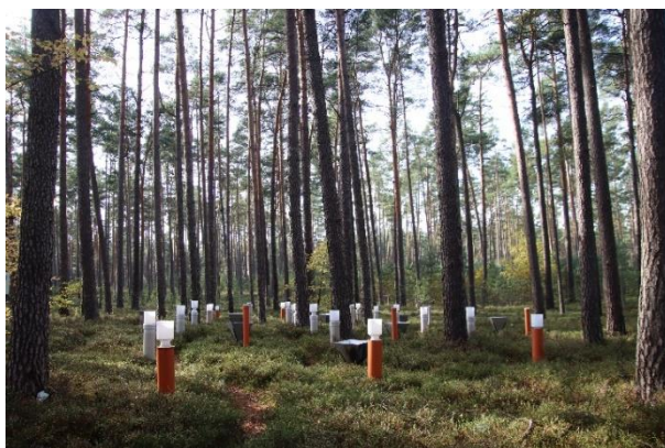
Figure 5-1: Throughfall samplers on a Level II plot (left) and open-field samplers on a neighboring meadow (right) in Schorfheide, Germany (Images: Berit Michler)
