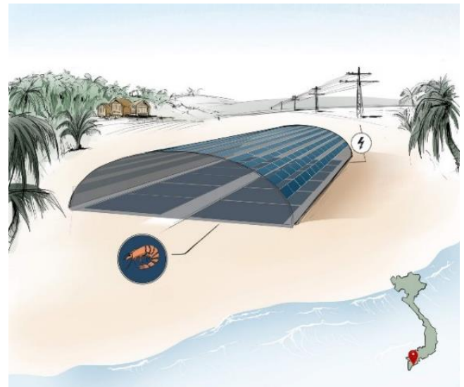
Figure 1: Schematic design of an Aqua-PV-facility with grid connection (Fraunhofer Institute for Solar Energy Systems (ISE), Freiburg, Germany).
