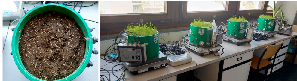
Figure 1. Experimental setup. (Left): Moist soil with the grass seeds. (Right): Four mini-lysimeters with DL6 data loggers mounted on scales after 18 days of initial growth.
