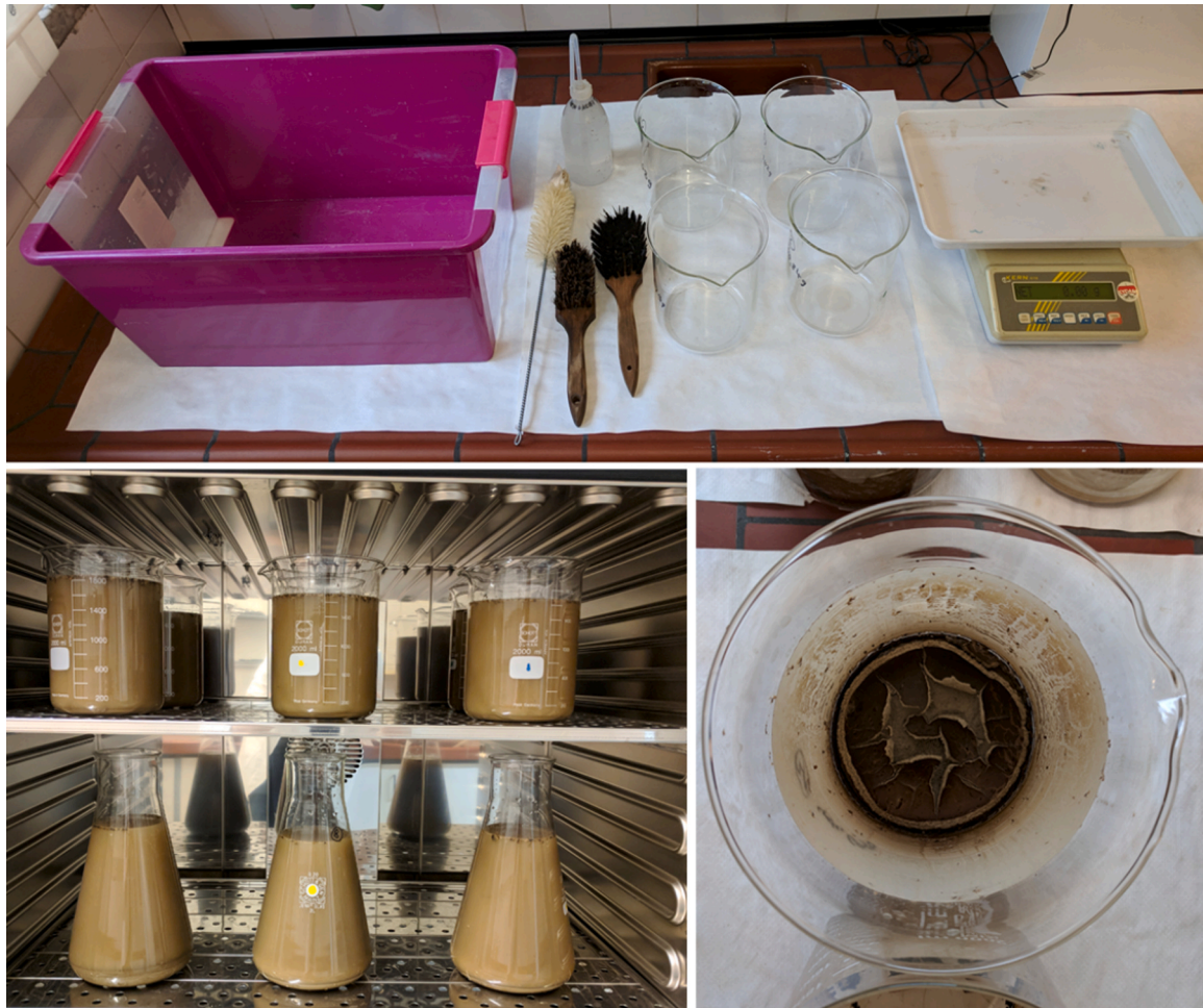
Figure A1. Cleaning of the sugar beets. (a) cleaning devices; (b) Soil-water-suspension in glasses placed in the oven to dry; Glass after drying.
