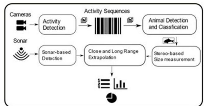
Figure 2: Documentation of the individual processing steps from data acquisition to final quantity estimation using the hybrid algorithm (Source: Thünen Institute / Gröger et al., 2024).
