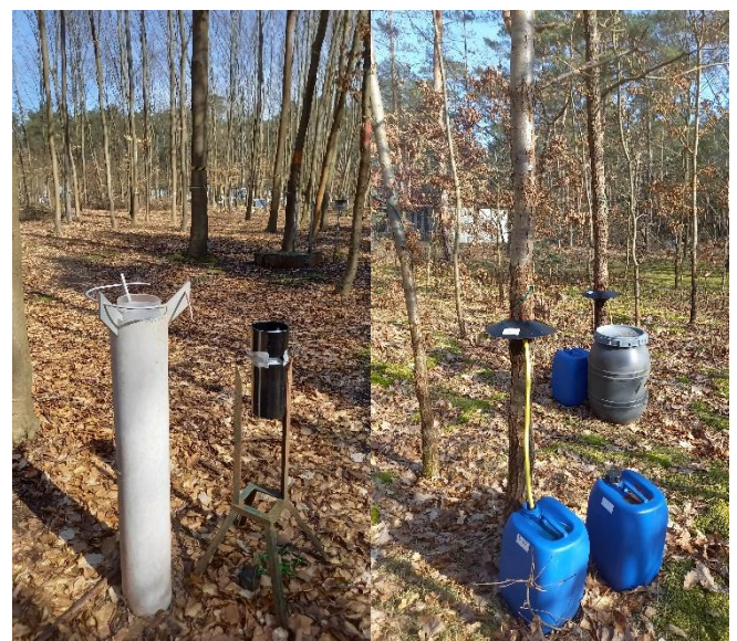
Figure 1: Precipitation samplers for throughfall (left) and stemflow (right) at the Britz Intensive Forest Monitoring Station (Source: A. Michel).
