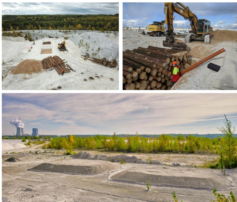
Fig. 5 In-ground storage of Norway spruce logs in a gypsum substrate on a gypsum storage area of MIBRAG in a former mining field south of Leipzig, Germany, top left: Aerial view of the storage site with both piles of 25 m 3 of Norway spruce wood each, top right: pile with slightly infested bark beetle wood, installation of the measuring equipment, bottom: pile covered with gypsum
