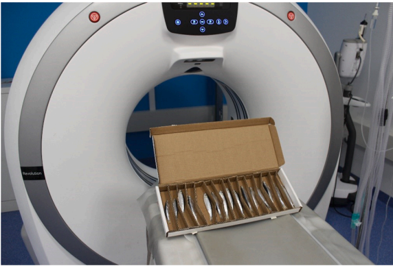
Fig. 1. TAC Philips Brilliance 16 P used for sprat scanning at JesiVet, Jesi (AN), Italy.
