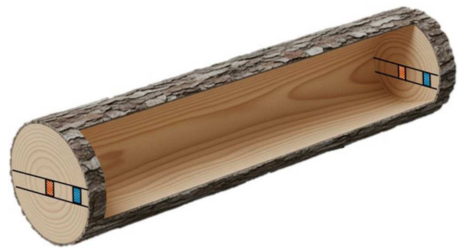
Figure 4. Sample design of gravimetric wood moisture content (MC) measurements on log sections prior and after dry storage. Red area marks the location of the heartwood test specimen and blue area marks the location of the sapwood test specimen.
