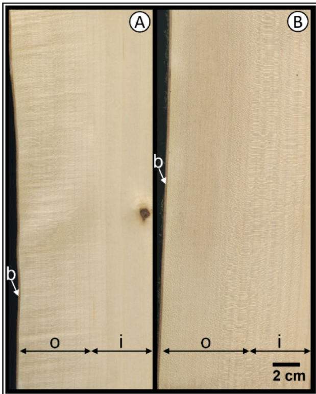
Fig. 2 Planed radial surfaces of 36-year-old sycamore maple, A =wavy grain, B =straight grain, b =bark, o =outer surface, i =inner surface
