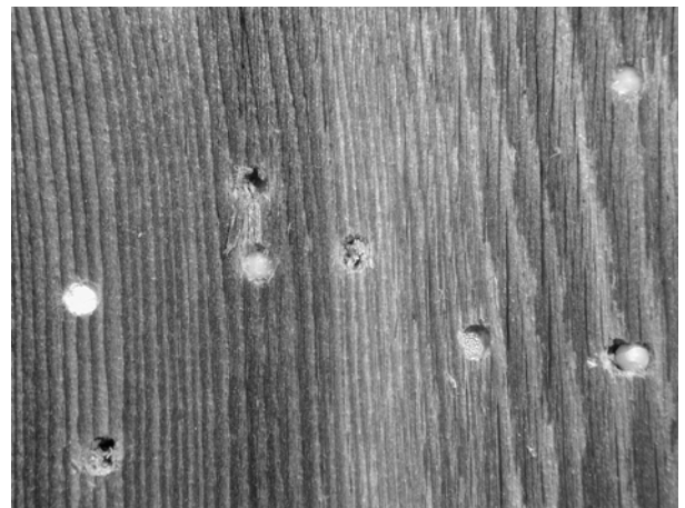
Fig. 4: Penetration of ECO-shot into the pinewood mount of the target
