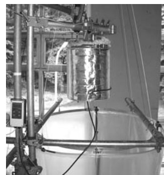
Figure 14: Heating chamber surrounding the JetCutter sitting on top of the 5 m tunnel
