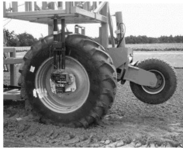
Figure 7 The view of the wheel equipped with the first monitoring system during field tests
